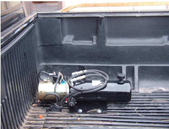
Power unit mounted in box
