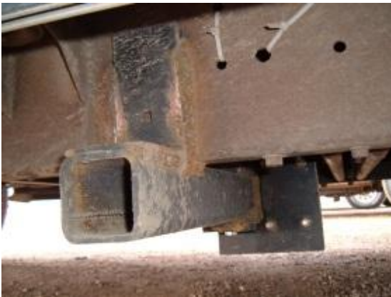
Cross member can be bolted or welded to frame.
