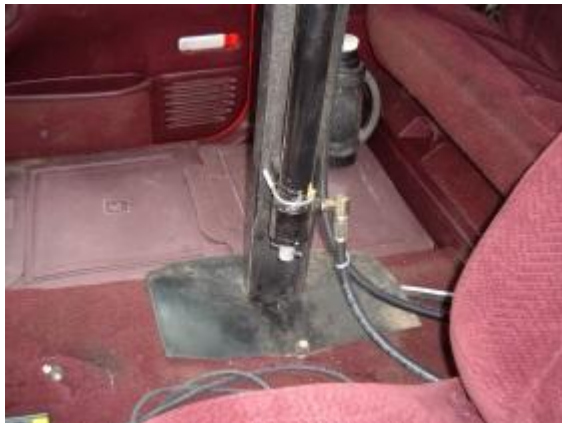
Inside mounting example, rubber dust seal.
